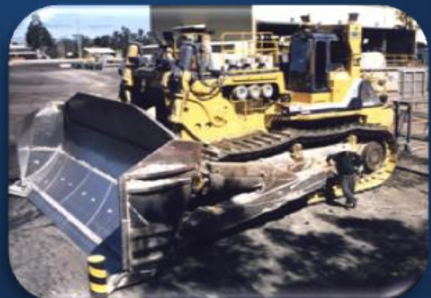
A Komatsu 575 - The world's largest & most powerful bulldozer. ( Note man leaning on blade arm )
