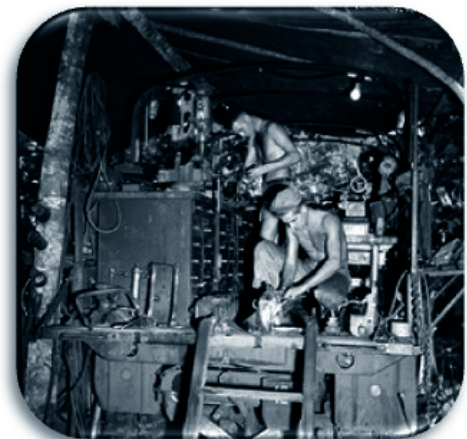
New Guinea in 1943. Mobile Machine Shop truck of the US Army with machinists working on automotive parts.
