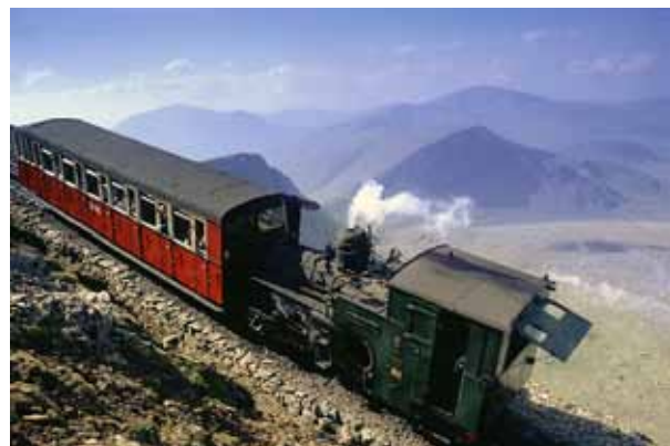
Engine # 6 "Padarn" works a 1 in 5 gradient on the Mt Snowdon rack railway , North Wales
